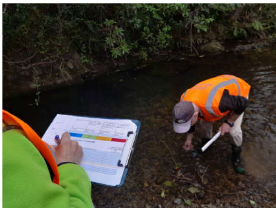
Recording pebble sizes to determine erosion risk in flood conditions.
